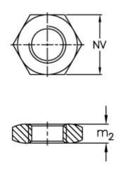
$\begin{array}{ll} m2 &= 1.8\\ Nominal size = M3\\ NV &= 5.50\\ Thread pitch = 0.50\\ Weight (g) &= 0.3 \end{array}$
